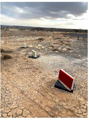
The aluminum sheaths will not corrode, and we anticipate them having a service life of 15 years. The UV and solvent resistant coatings ensure durability which allows for rugged outdoor use. Conspicuity-grade material like this is typically 6 or 7 times more reflective than a comparable color in an engineering-grade reflective tape since prism technology is used instead of glass beads, which greatly increases the visible range of the runway markers.
