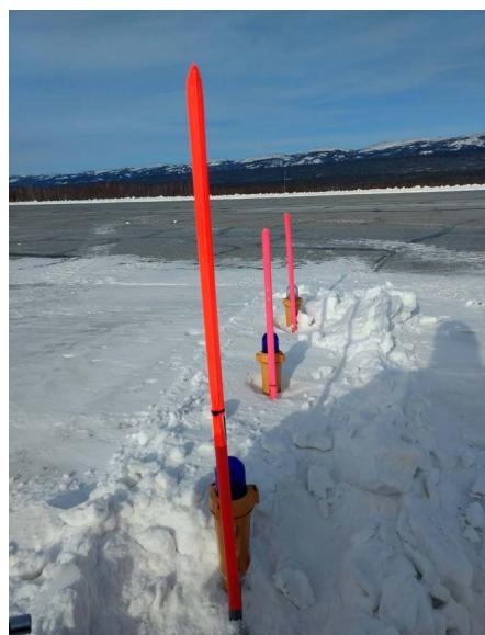
*The iSeries RELMs have different lengths: 18", 24" and 36" depending on the snow depth, offering an easy installation to do within minutes.*
